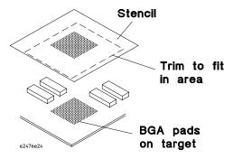
**3** Once the stencil is trimmed to the proper size, remove its adhesive back. Carefully align the stencil on the target board and press it down. The stencil is properly aligned when all stencil holes are completely filled with PCB pads, or when the PCB pads are all centered in the stencil holes. If misaligned, lift the stencil, realign, and press it down again.
